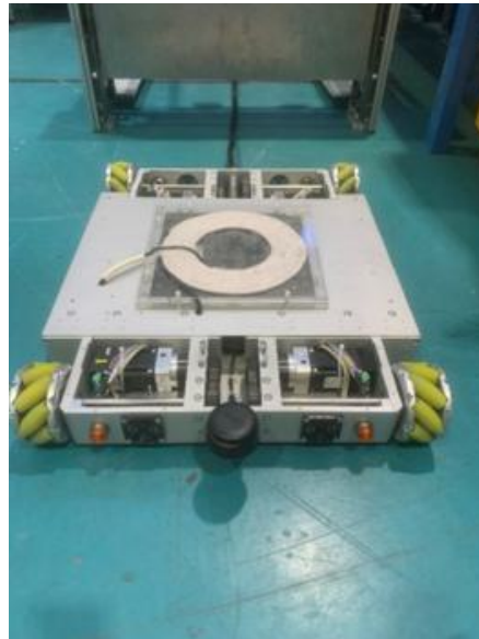
The tethered robotic platform designed for wireless charging EV of disabled drivers. Transmitting coil seen above the robot. Lidar sensors for navigation are seen in front of the robot. Tether cable for supplying electricity and communication is seen behind the robot.
